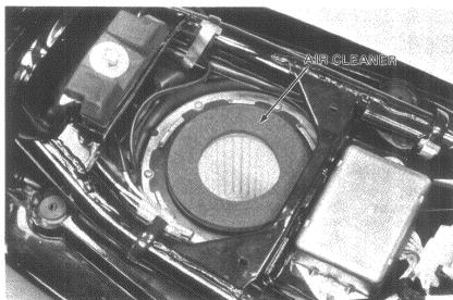
Clean the air cleaner element by tapping it lightly to loosen dust. Remove the remaining dust with compressed air.
