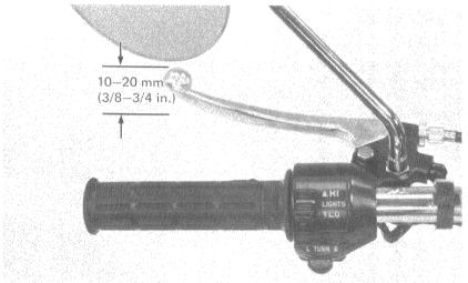
Major adjustments should be made using the adjuster located at the clutch housing. Loosen the lock nut and turn the clutch cable adjusting nut.
