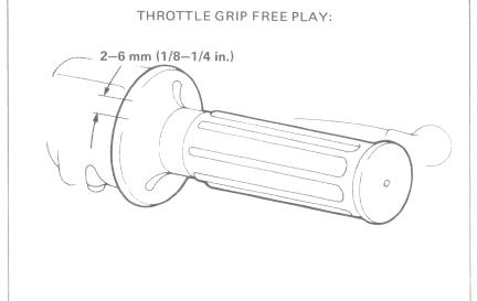
Throttle grip free play can be adjusted at either end of the throttle PULL cable. Major adjustments must be made at the lower adjuster. Adjust by loosening the adjuster lock nut and turning the adjuster. Tighten the locknut. Minor adjustments must be made at the upper adjuster.
